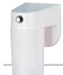
Lexan Cylinder with Photoelectric Sensor Energy Saver 77-749 White Requires (1) 13W Quad tube GX23-2 Base max. Dimensions: Diameter 4", Height 8", Extension 6"
